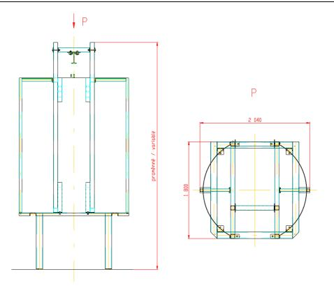
Brushing device is used for pork slaughter. It functions to pig's cleaning at bleeding railway before coming to scalding tube. Device is made out of stainless profile and plastic boards. There are locate two rotating brushes, which are driven by elektric gear-boxes Nord. Showering is started up automatically with passing hanging carcass.
